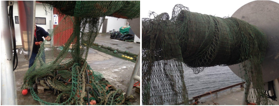
Photographs above: During the workshop at the Port of Smögen (FF Norden), the project team used an electric net roller for raising the DFG material to a suitable work height.
