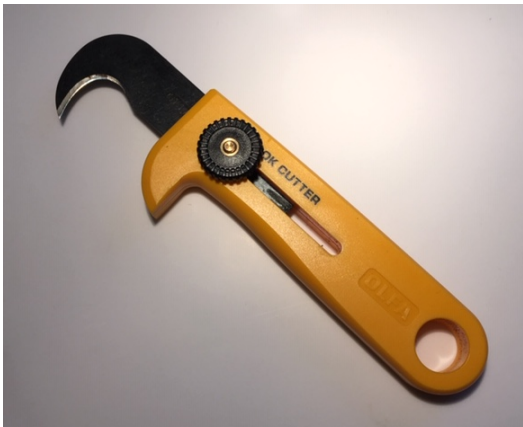
Photograph above: A hooked blade cutter works well for the initial dismantling of some types of entangled DFG
