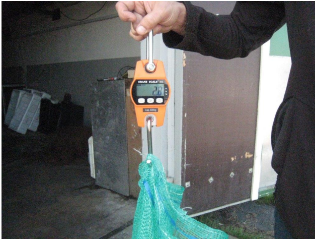
Photograph above: Light polypropylene woven bags and a digital crane scale were used for weighing of cleaned and sorted material.
