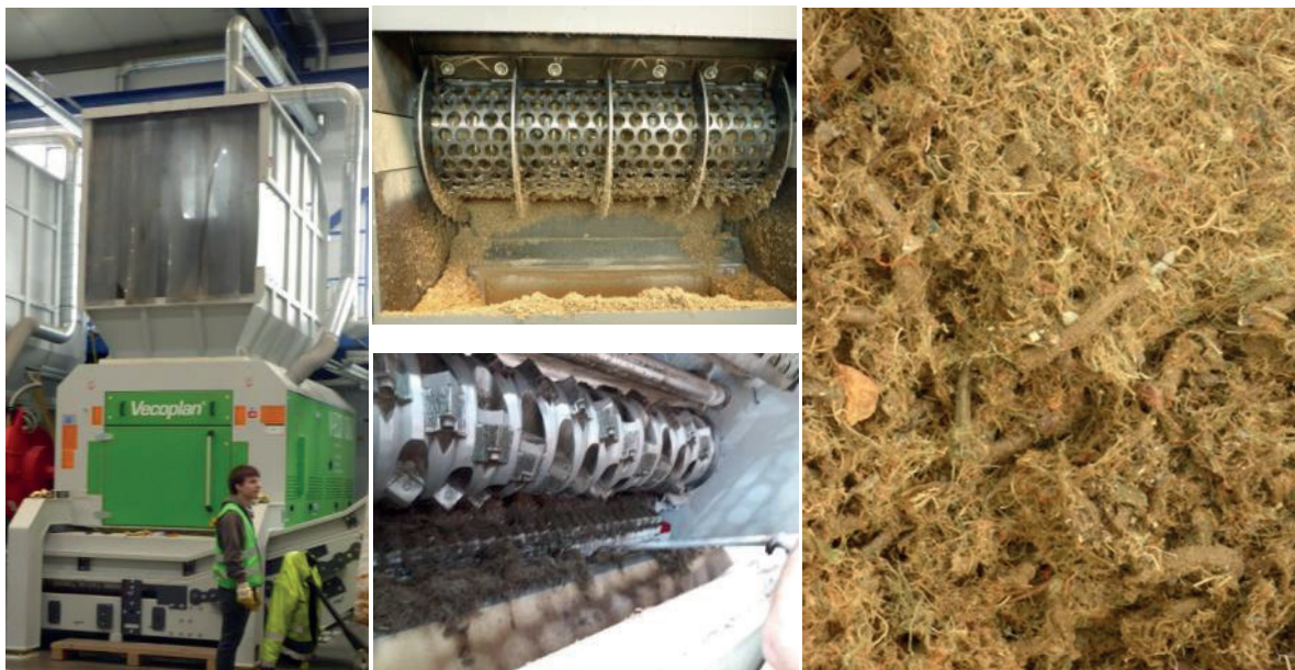
Fig. 16 Industrial shredder with anti-blocking system used in MARELITT Baltic trials to shred net fibres to 2-4cm length (left, at Vecoplan AG); rotor with counter-blade triangles and sieve (middle), and gillnet fibres with lead fragments after shredding. This material can be used for alternative thermal processing such as steam reforming (evaporation).
