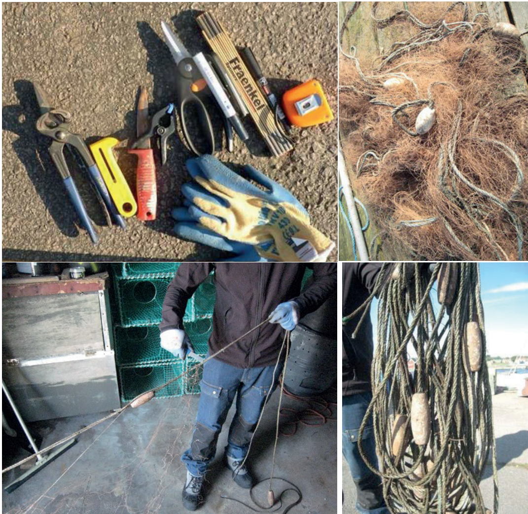
Fig. 10 Pre-processing of retrieved gillnets during MARELITT Baltic trials in Karlskrona, Sweden: a) Tools used for cutting and measuring, b) entangled gillnet with float line and sink line, c) removal of float line from polyamide netting, d) extracted float line which can be re-used (all images © Marek Press).
