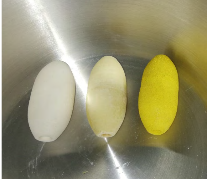
Fig. 42. Float No. 3 "traditional" 3D print on the left, casting inside, casting covered with yellow acrylic varnish on the right.
