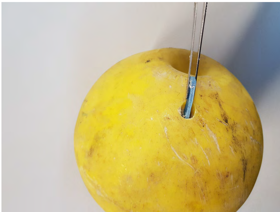
Fig. 47. Installation of RFID tag impregnated with CW5620 Arathane blue resin, to the round float.
