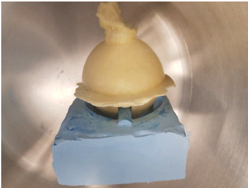
Fig. 39. Casting of polyurethane foam removed from a silicone mold (visible excesses)
