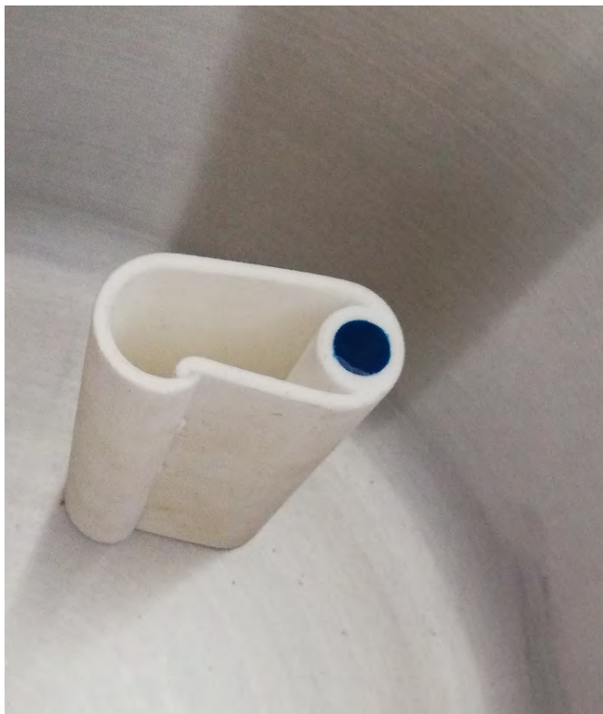
Fig. 46. Printed prototype of float No. 5 "clip" Source: Own study
