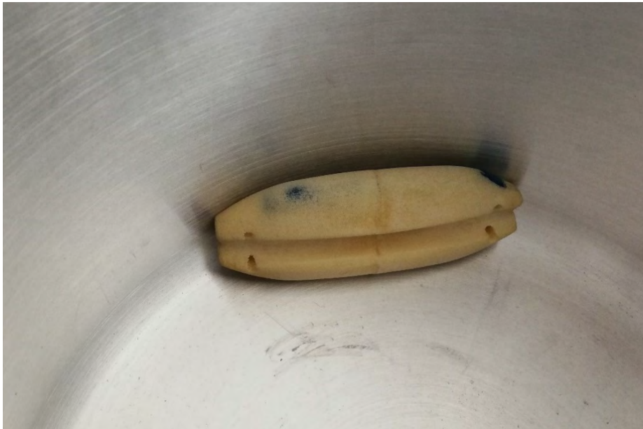
Fig. 45. Polyurethane casting of float No. 4 "fish" with installed UHF RFID tag (visible blue resin impregnating the tag) Source: Own study
