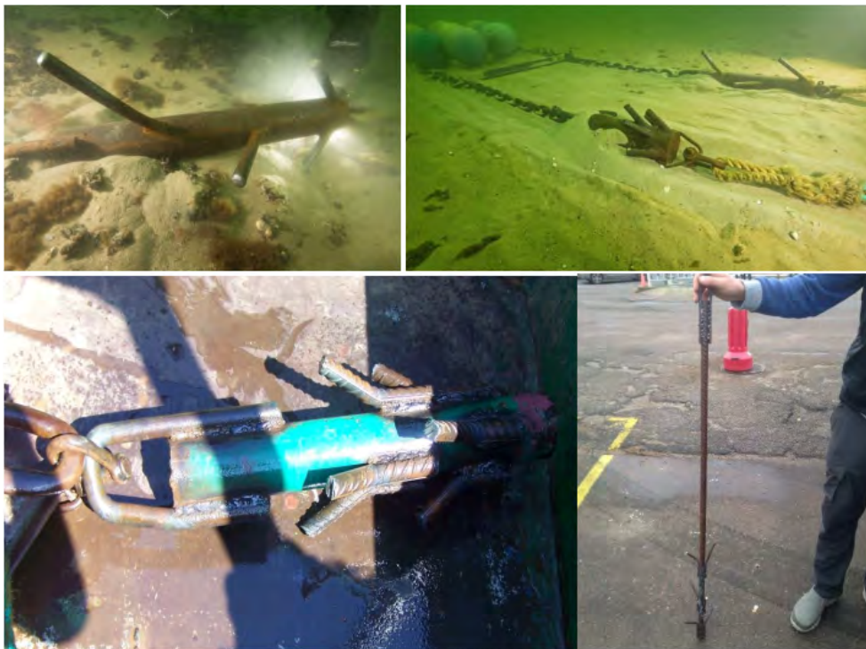
Figure 14. Upper right and left: searching devices used in Germany, (© Christian Howe). Lower left: searching device used in Poland. Lower right: searching device used in Estonia.
